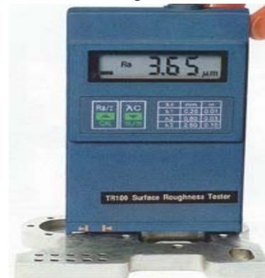
Fig.4.5: Portable Surface Meter TR100
