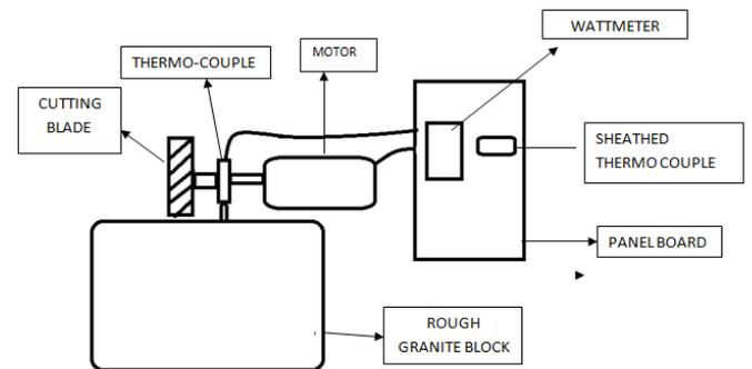
Fig.4.1: Showing Line Diagram of Experimental Set Up
